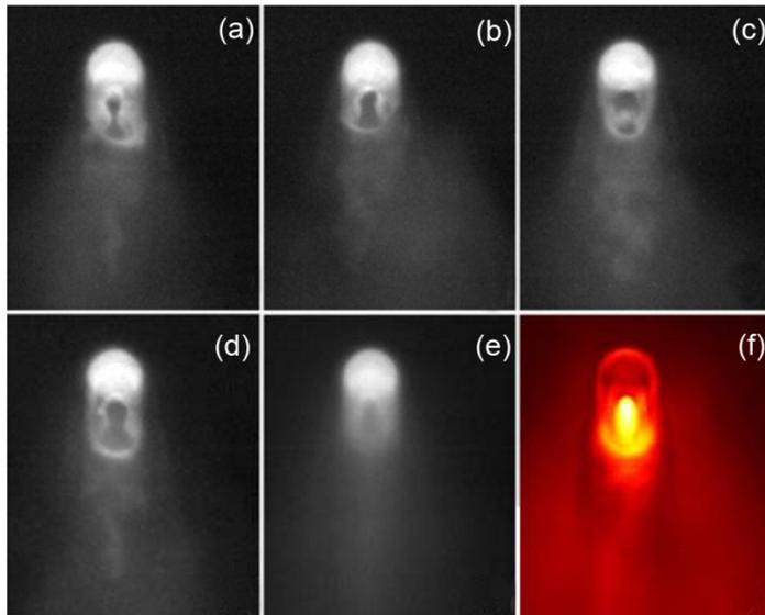
**Figure 1.3:** From (a) to (d), sample images of a sequence acquired at a frame rate of 3 *kHz* are shown. Pictures (e) and (f) represent respectively the mean grey value calculated over 100 images and the corresponding standard deviation [20]. Picture (f) was rescaled from 0 to 255 digits and a different colormap was used to enhance the contrast of the FPH area.
