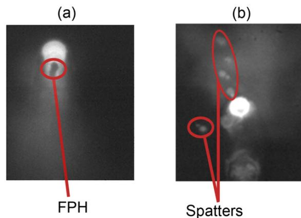
**Figure 1.2:** Two typical LBW coaxial process images. (a) shows an example of FPH, while spatters are visible in (b).
