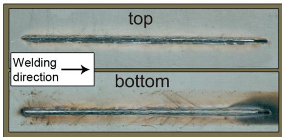
**Figure 1.1:** Uncontrolled full-penetration weld of two 0.7 mm thick zinc-coated steel sheets in an overlap joint with 0.1 mm gap. The process was performed at 9 m/min by using a constant laser power of 5.5 kW with 10% power as factor of safety [21].
