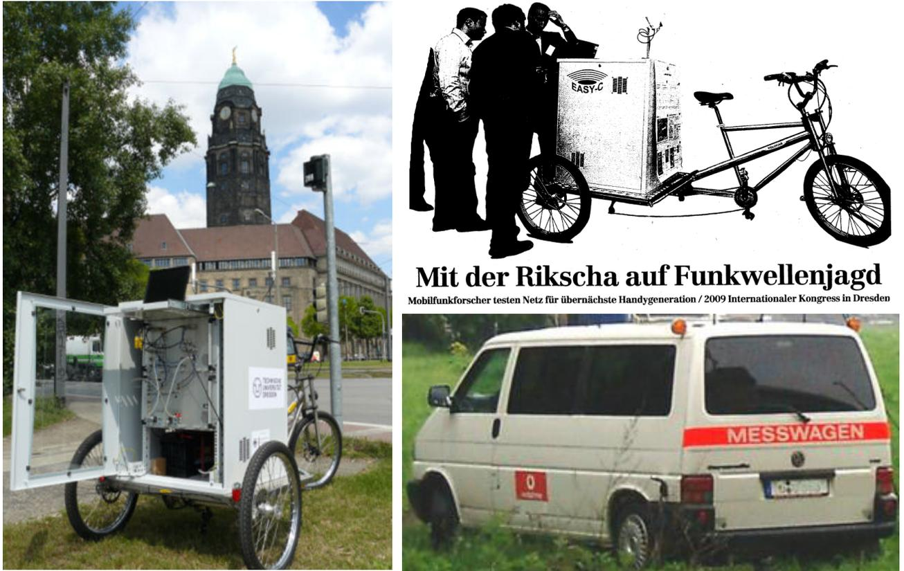
Figure 1.1: The mobile terminal measurement equipment.
